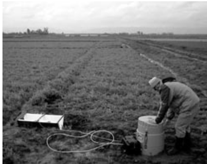
SAFS research assistant Aaron Ristow checks datalogger monitoring surface runoff in vetch cover crop plot.
